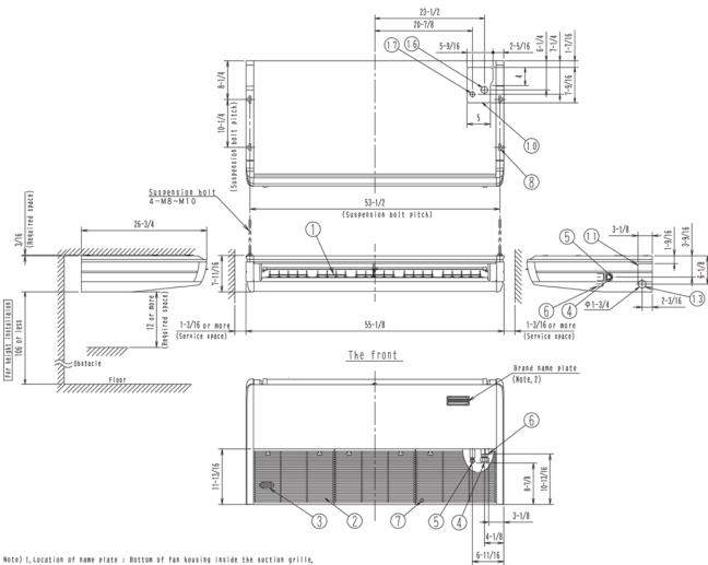
Note) |, Location of name plate : Bottom of fan housing inside the suction grille, 2, In case of using a wireless remote controller, this position will be the signal receiver, Refer to the drawing of wireless remote controller in detail.
